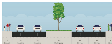
Existing Typical Section
