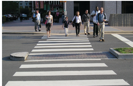
Median Nose and Curb Extensions
