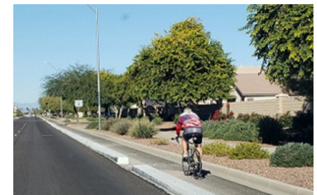
Median Bicycle Lane with Concrete Buffer
