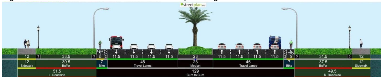
Figure 12. Mixed Traffic with Limited Bus Stops Design Plan
