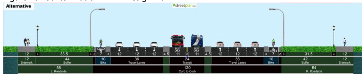
Figure 15. Center Platform BRT Design Plan
