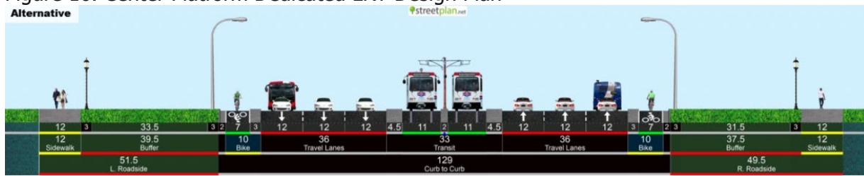
Figure 16. Center Platform Dedicated LRT Design Plan
