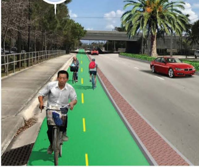
4 lane divided with landscaped median 10' travel lanes with existing 7' sidewalks 8' two-way protected bike lane with 2' raised separator
