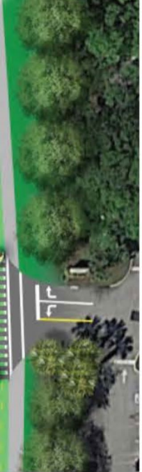
4 lane divided with landscaped median 10' travel lanes with existing 7' sidewalks 8' two-way protected bike lane with 2' raised separator
