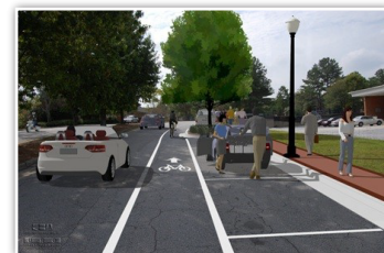
Potential Countermeasure: Lane Eliminations/Narrowing
